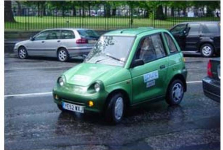
The REVA electric car modified by SiGen to include a 1 kW fuel cell as a battery range-extender. The vehicle is operated by the PURE partnership and fuelled by hydrogen generated by the PURE wind-hydrogen system.
