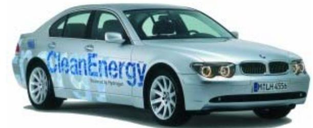
BMW's hydrogen powered 7 series incorporates hydrogen ICE technology and liquid hydrogen storage
