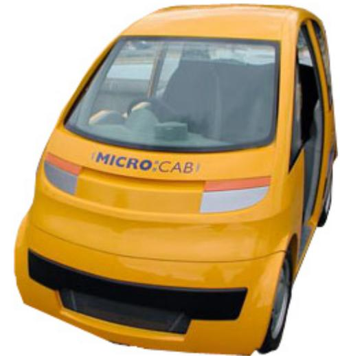
Microcab – small fuel cell passenger and delivery vehicles
