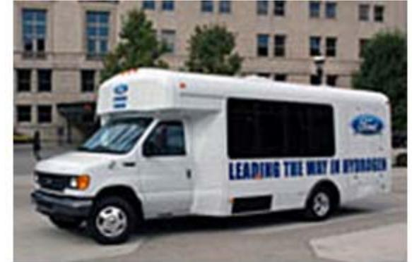
Ford E450 shuttle bus with hydrogen ICE
