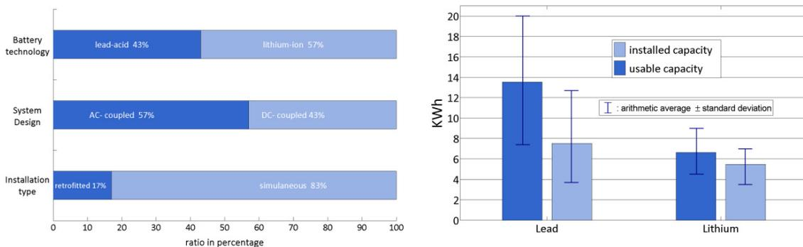
Fig. 1. (left) Overview about typical system configurations of the registered PV Battery Systems (right) Average installed and usable capacity of the registered PV Battery Systems
