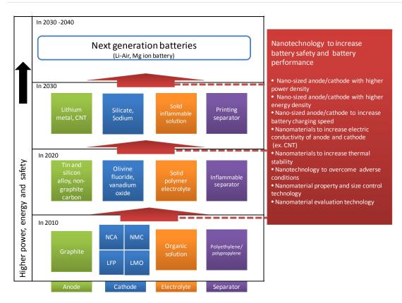
Figure 23. Lithium-ion battery road map and nanotechnology
