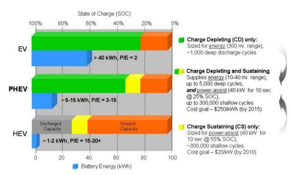
Figure 1. Battery performance requirement by vehicle application
